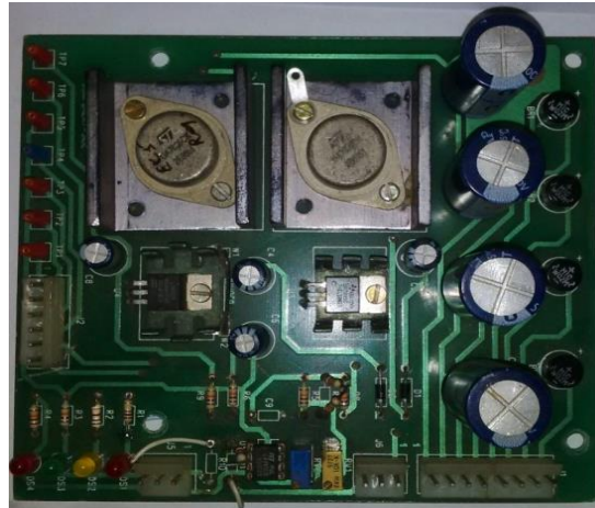
Fig 3. (c) Power interface board
